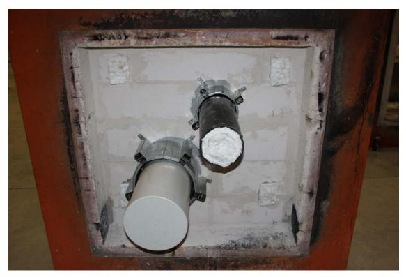
PHOTOGRAPH 1 – EXPOSED FACE OF SPECIMENS PRIOR TO TESTING
