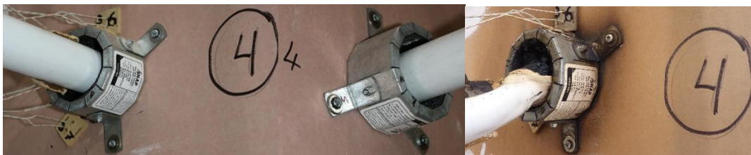
Photo 6: Penetration 4, left to right, unexposed, exposed and unexposed post test
