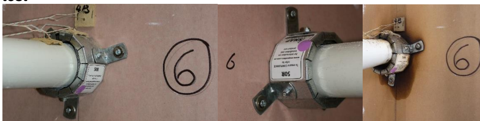
Photo 8: Penetration 6, left to right, unexposed, exposed and unexposed post test
