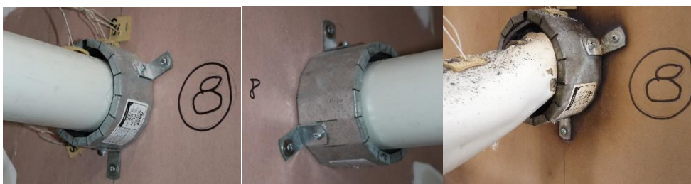
Photo 11: Penetration 9, left to right, unexposed, exposed and unexposed post test
