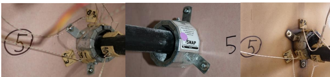
Photo 7: Penetration 5, left to right, unexposed, exposed and unexposed post test
