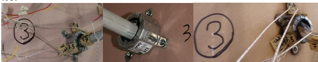
Photo 5: Penetration 3, left to right, unexposed, exposed and unexposed post test
