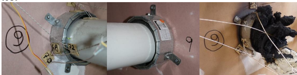
Photo 11: Penetration 9, left to right, unexposed, exposed and unexposed post test
