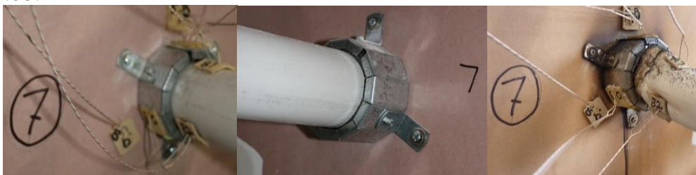
Photo 9: Penetration 7, left to right, unexposed, exposed and unexposed post test
