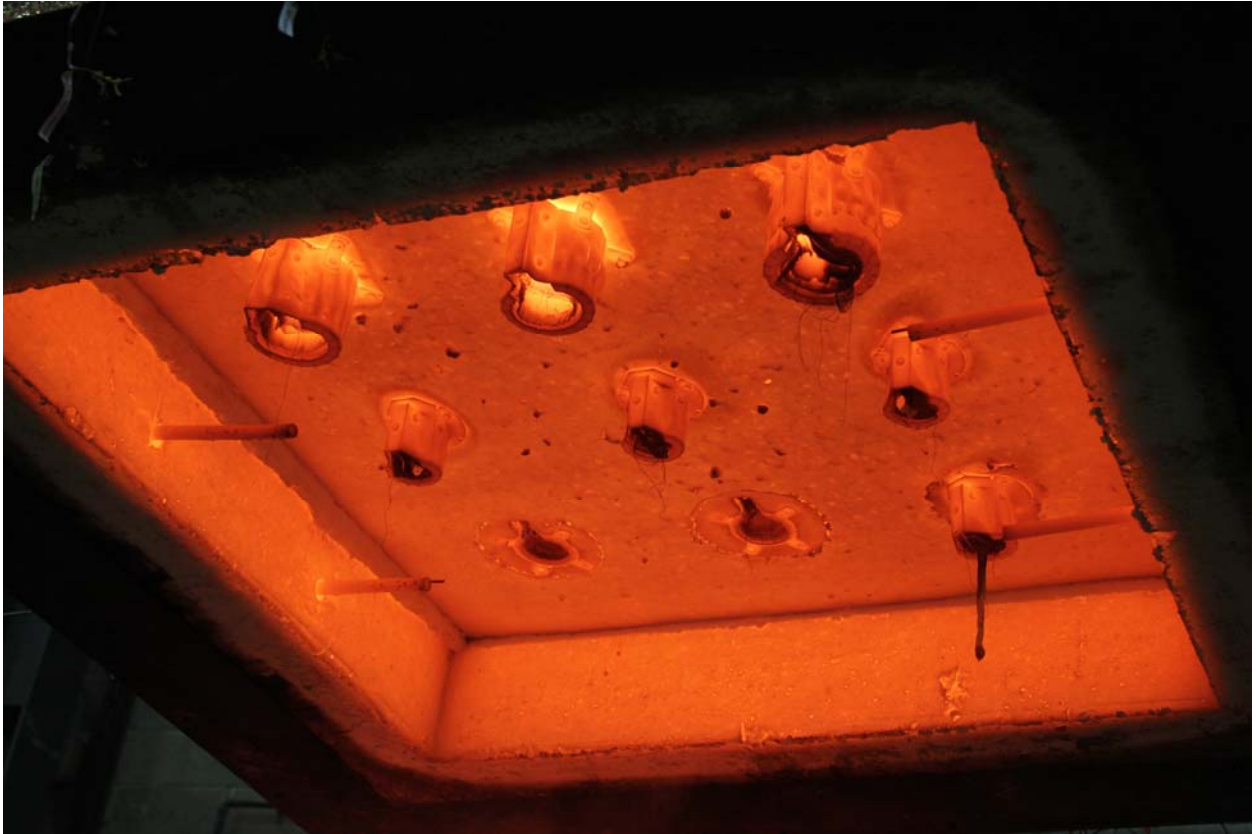
PHOTOGRAPH 6 – EXPOSED FACE OF SPECIMENS AT CONCLUSION OF TESTING
