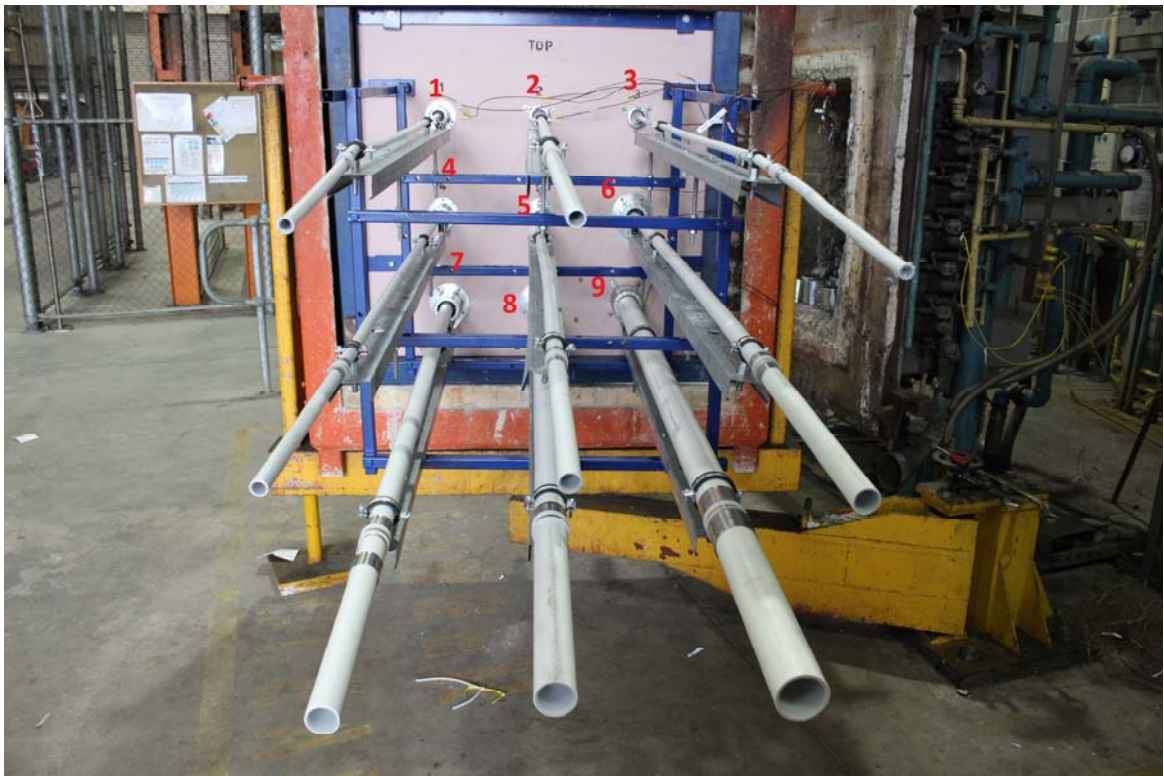
PHOTOGRAPH 1 – UNEXPOSED FACE OF SPECIMENS PRIOR TO TESTING
