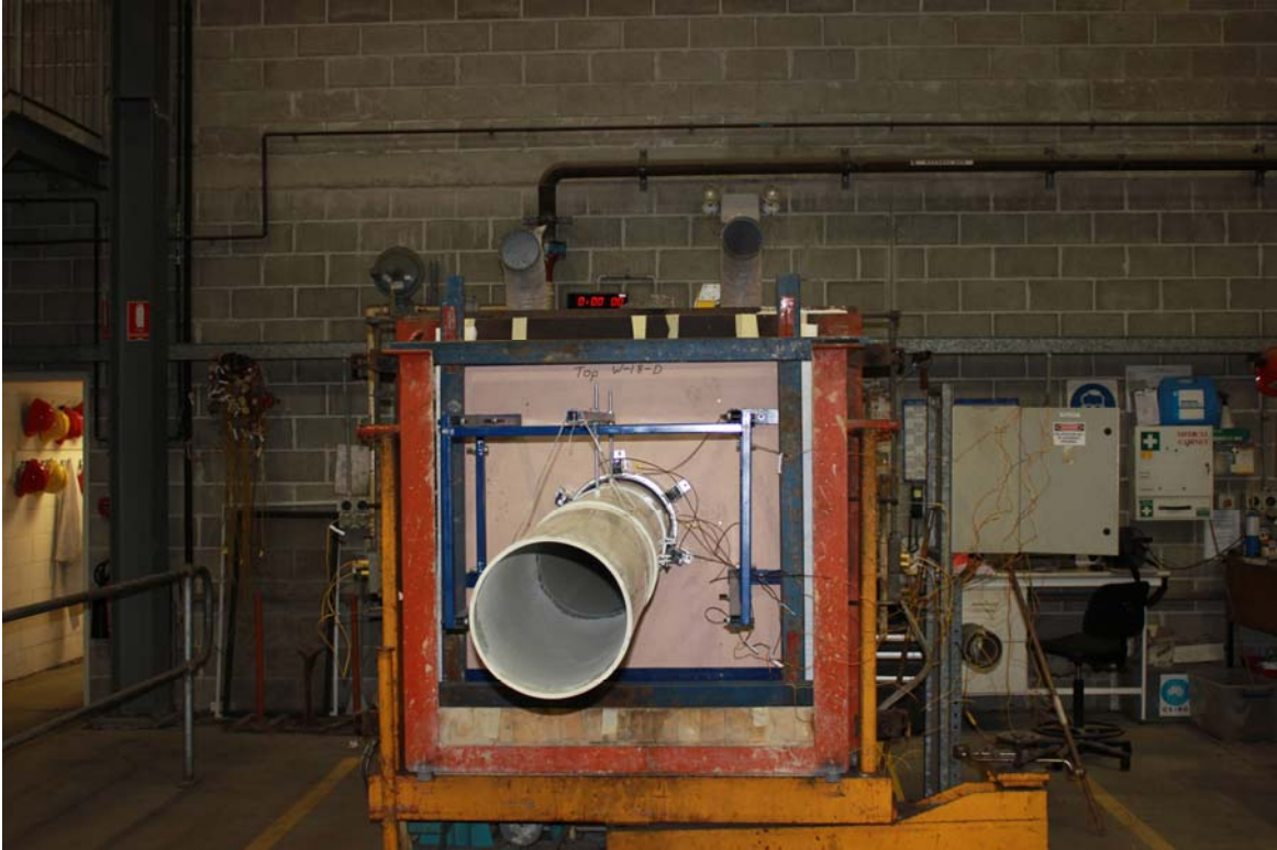
PHOTOGRAPH 2 – UNEXPOSED FACE OF SPECIMEN PRIOR TO TESTING
