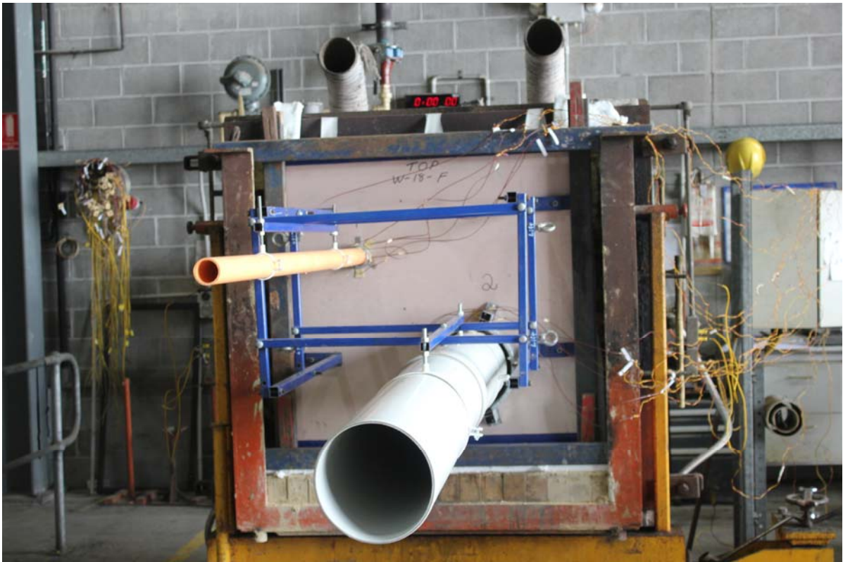
PHOTOGRAPH 2 – UNEXPOSED FACE OF SPECIMENS PRIOR TO TESTING
