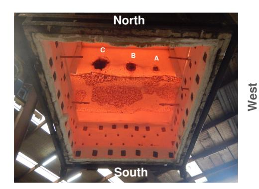
Figure 16 Exposed face of the specimen at the end of test
