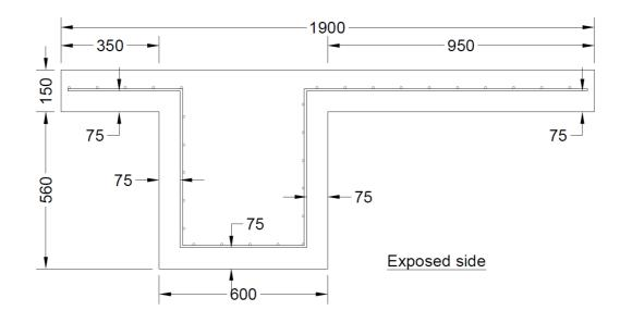
Figure 2 Cross-section of the test specimen (A-A)
