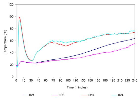
Figure 11 Penetration system B – temperature vs time
