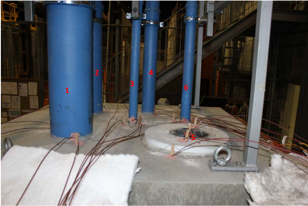
PHOTOGRAPH 2 – UNEXPOSED FACE OF SPECIMENS PRIOR TO TESTING
