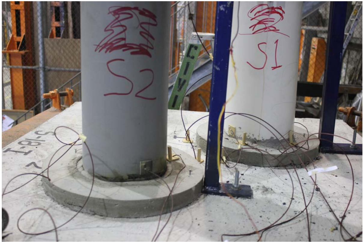
PHOTOGRAPH 7 – SPECIMENS AFTER 180 MINUTES OF TESTING
