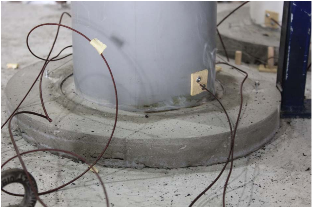
PHOTOGRAPH 5 – BASE OF SPECIMEN 2 AFTER 122 MINUTES OF TESTING
