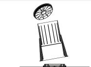
Pour concrete. Snap cast-in Fire Collars are approved for use in concrete slabs of a range of thicknesses (see website: www.snapcollars.com.au for tested systems).
