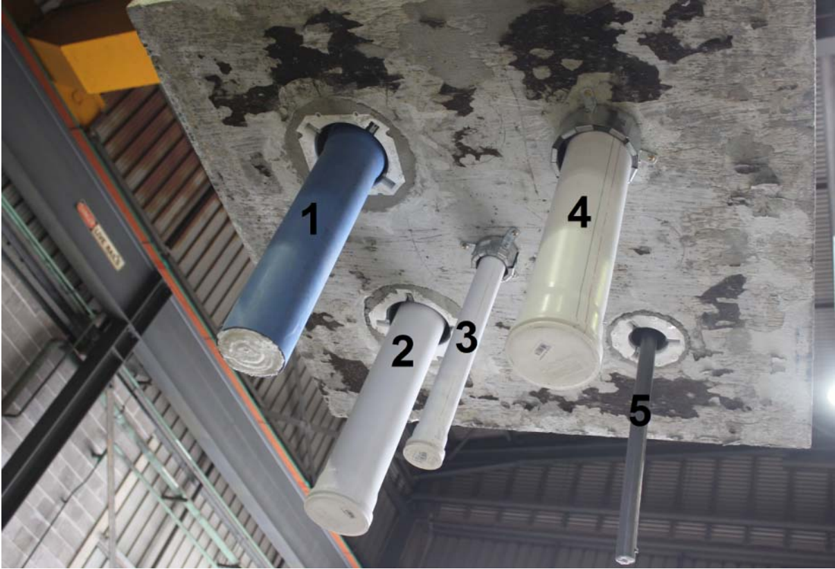
PHOTOGRAPH 1 – EXPOSED FACE OF SPECIMENS PRIOR TO TESTING
