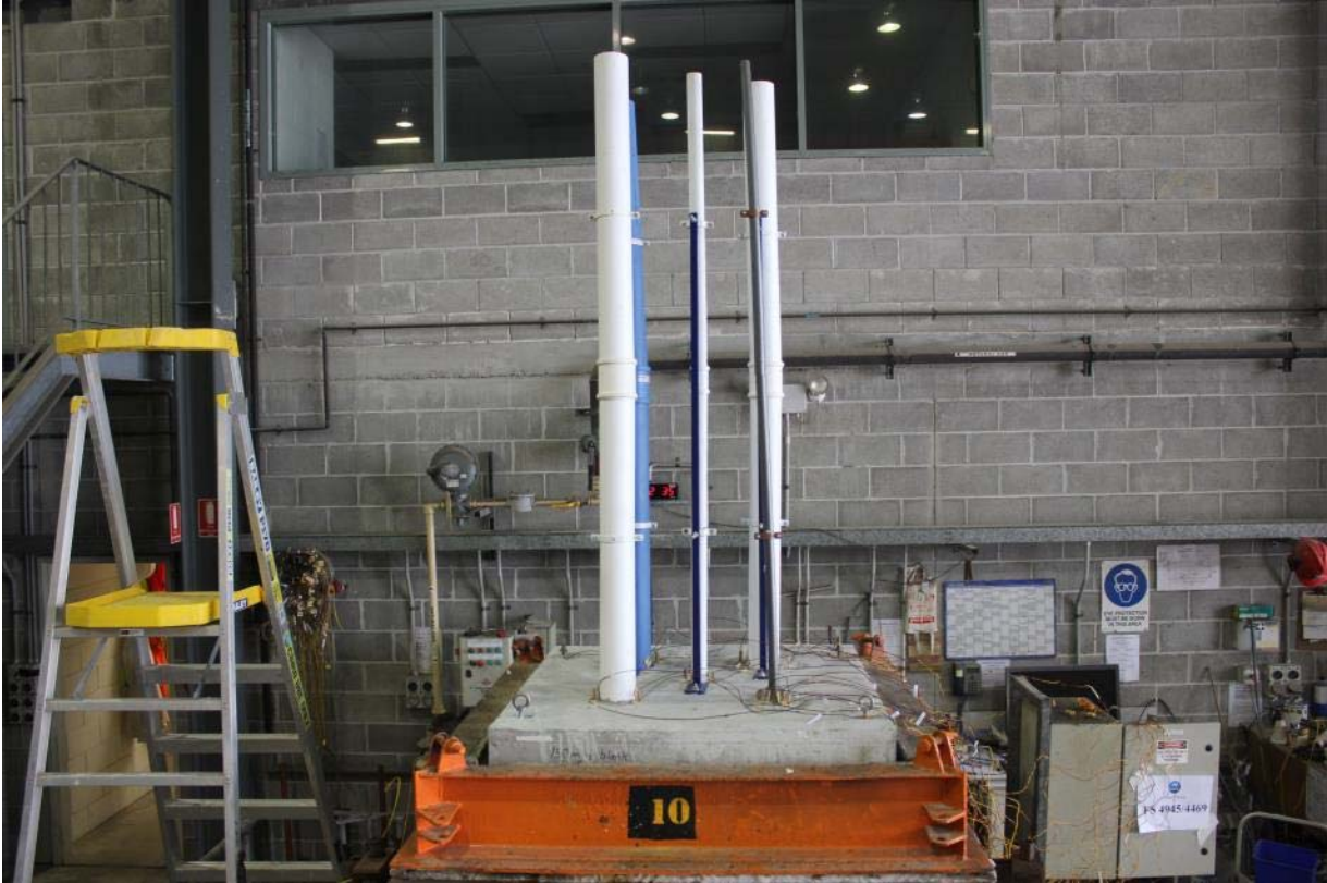
PHOTOGRAPH 2 – UNEXPOSED FACE OF SPECIMENS PRIOR TO TESTING
