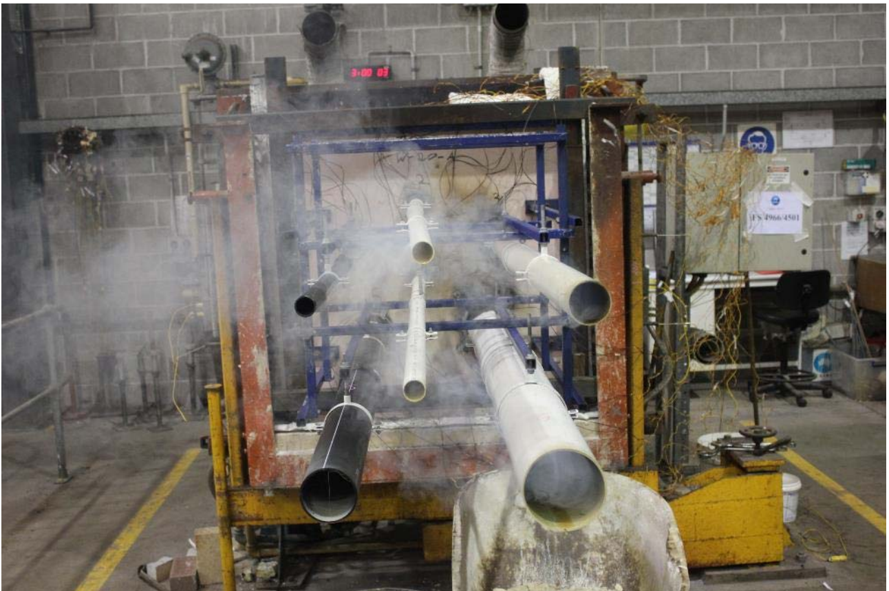
PHOTOGRAPH 16 – SPECIMENS AFTER 180 MINUTES OF TESTING
