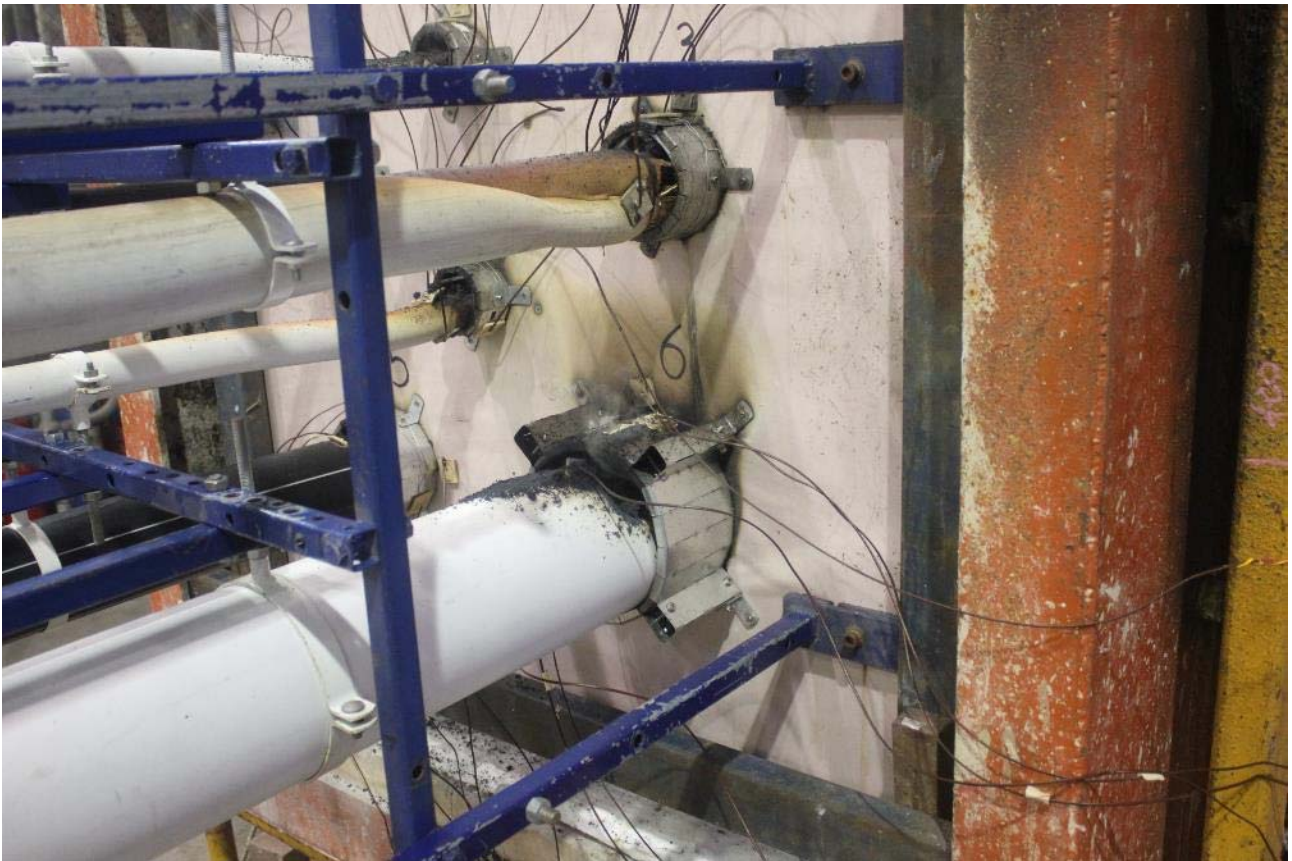
PHOTOGRAPH 15 – SPECIMENS AFTER 154 MINUTES OF TESTING
