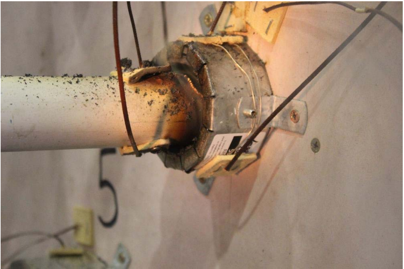
PHOTOGRAPH 11 – SPECIMEN 5 AFTER 105 MINUTES OF TESTING
