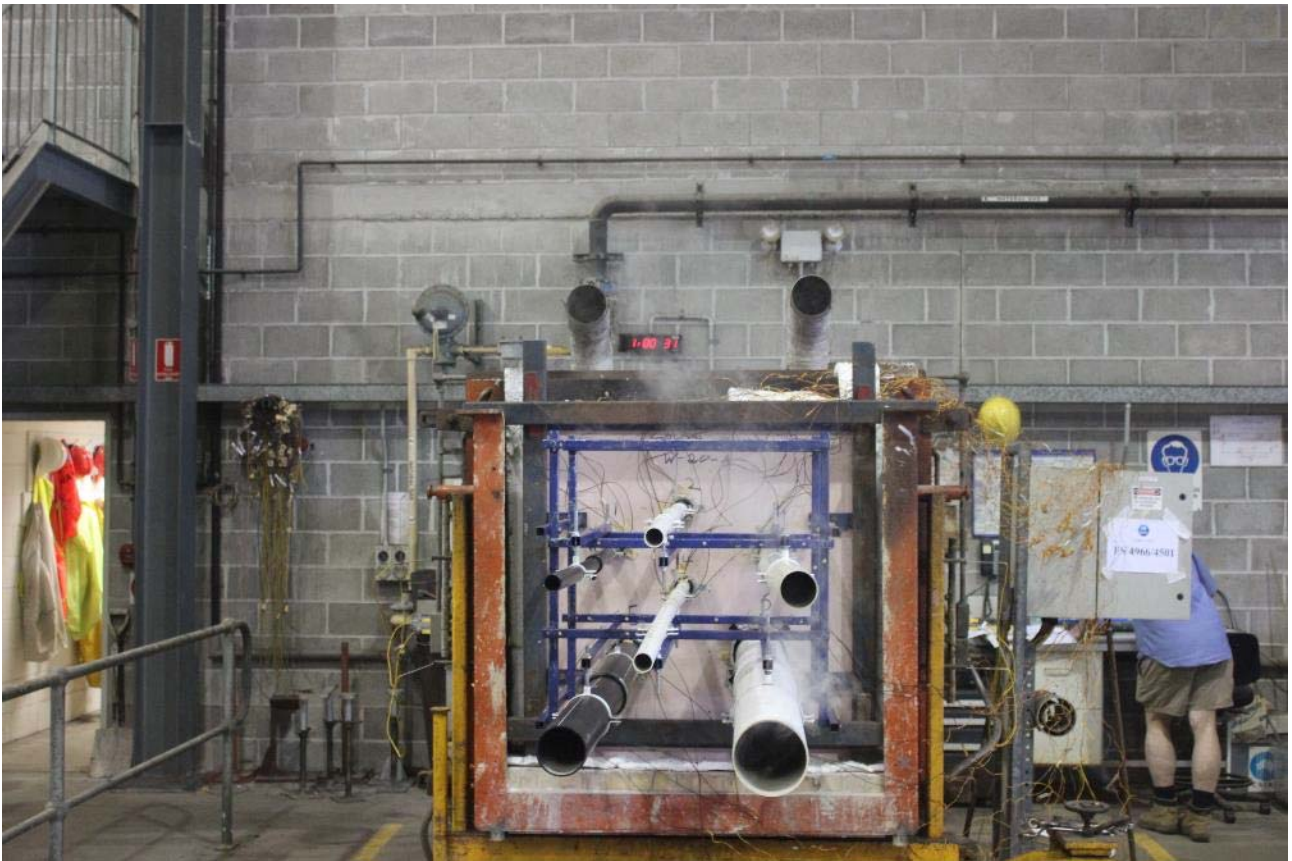
PHOTOGRAPH 7 – SPECIMENS AFTER 60 MINUTES OF TESTING
