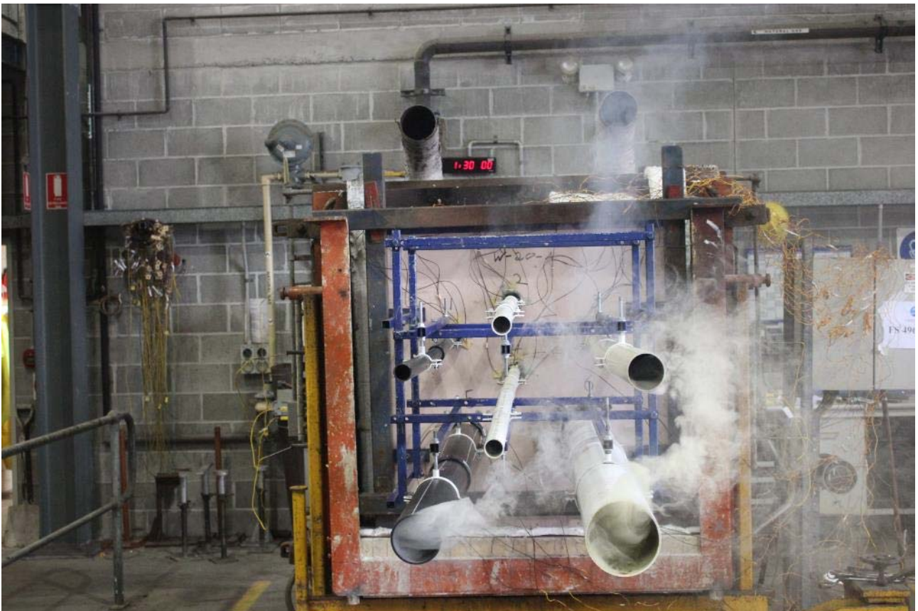
PHOTOGRAPH 8 – SPECIMENS AFTER 90 MINUTES OF TESTING
