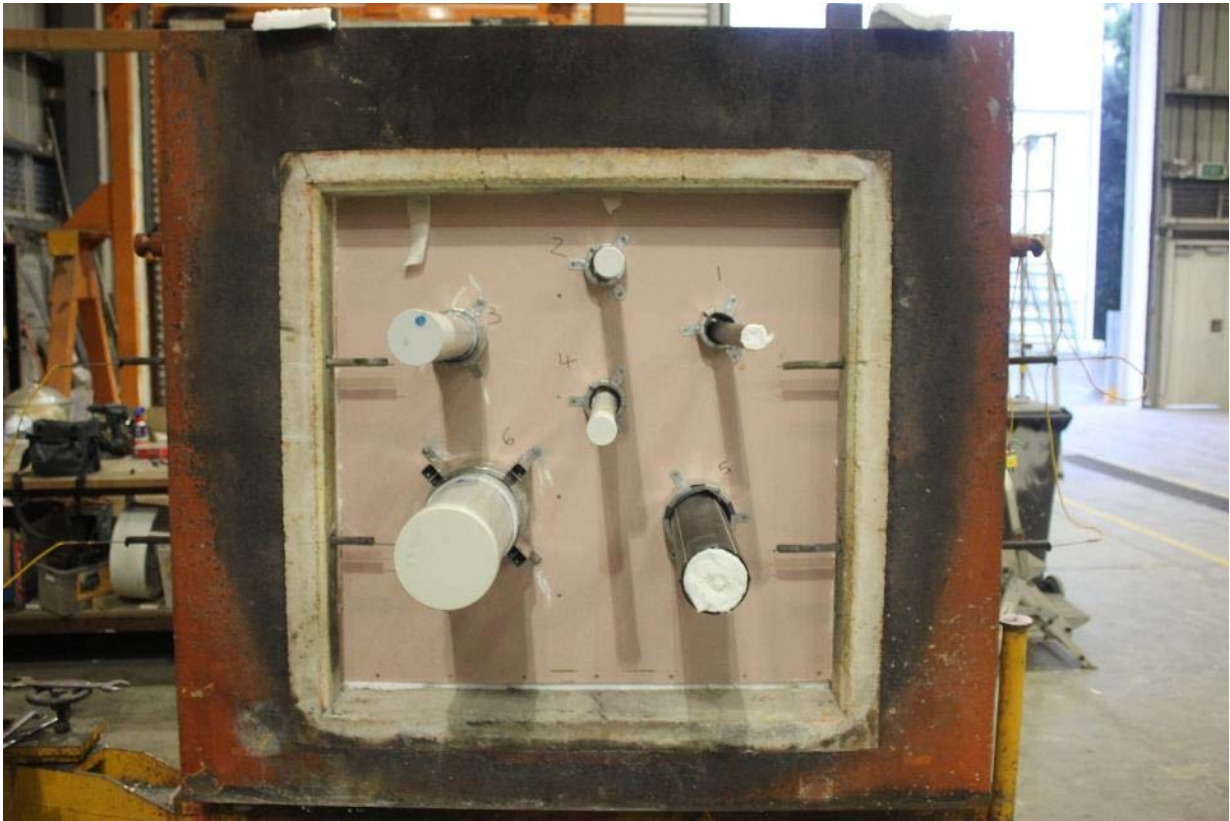
PHOTOGRAPH 1 – EXPOSED FACE OF SPECIMENS PRIOR TO TESTING
