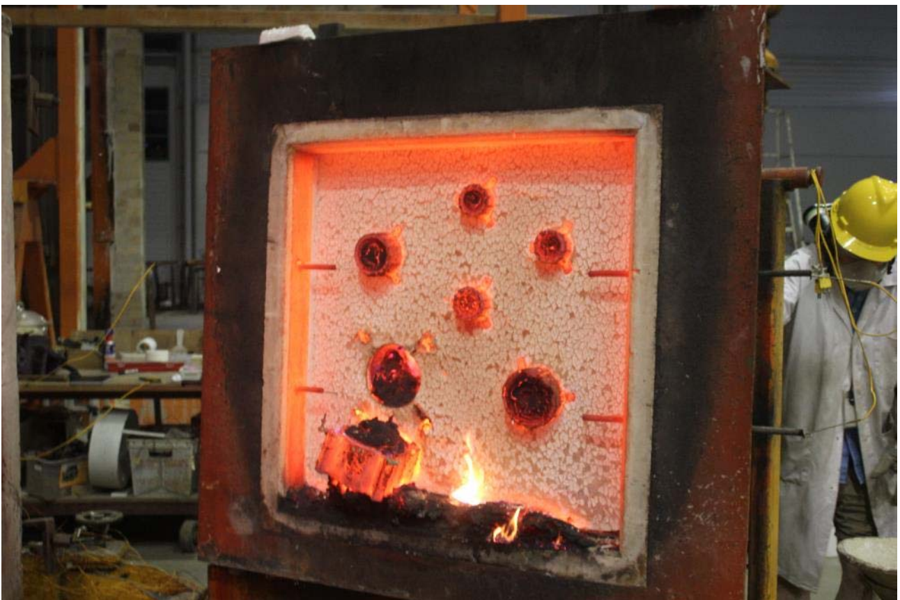
PHOTOGRAPH 18 – EXPOSED FACE OF SPECIMENS AT CONCLUSION OF TESTING
