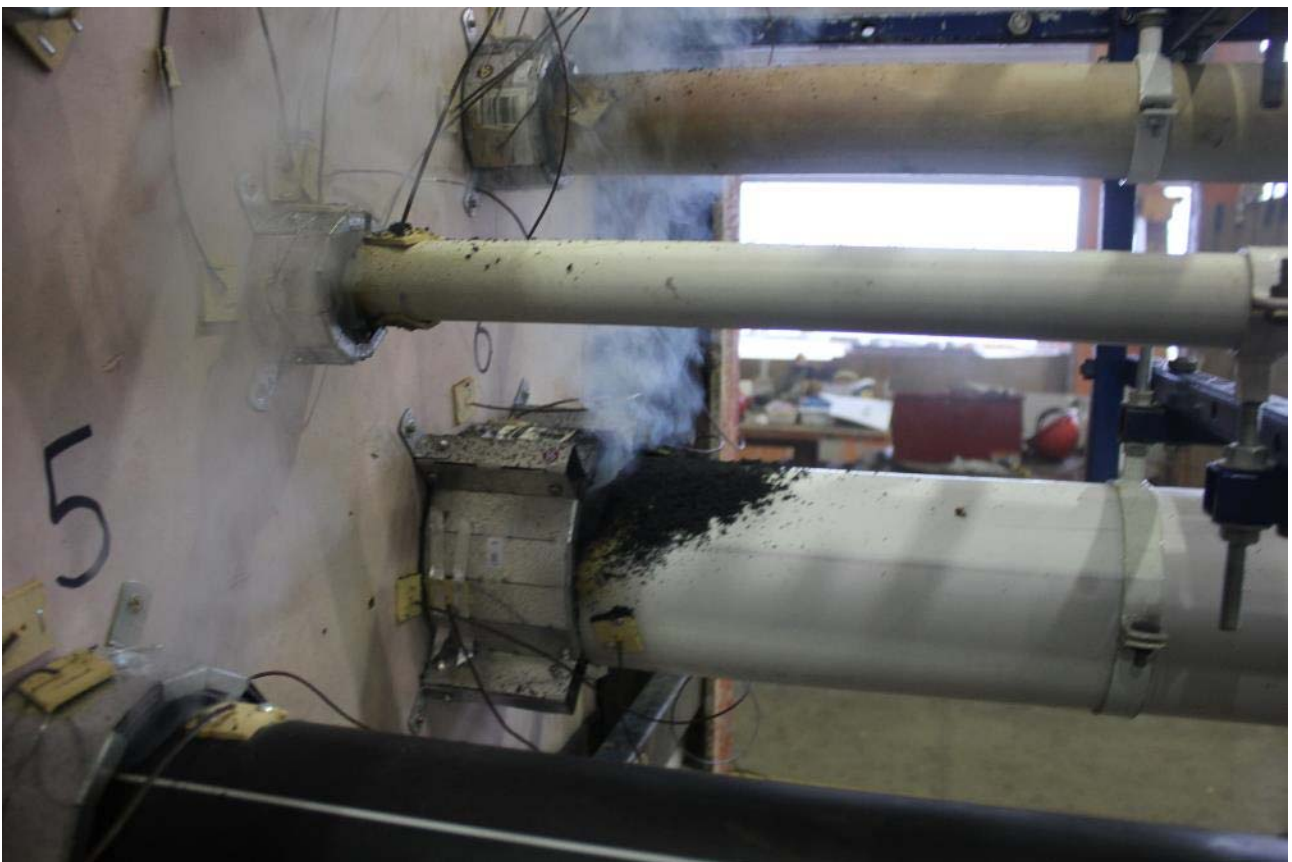
PHOTOGRAPH 10 – SPECIMEN 6 AFTER 100 MINUTES OF TESTING
