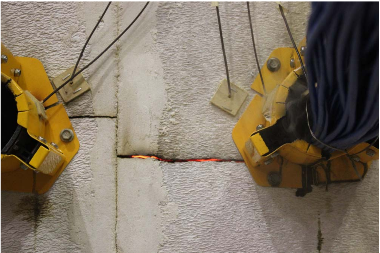
PHOTOGRAPH 10 – THE WALL ADJACENT TO SPECIMENS 3 AND 4 AFTER 97 MINUTES OF TESTING
