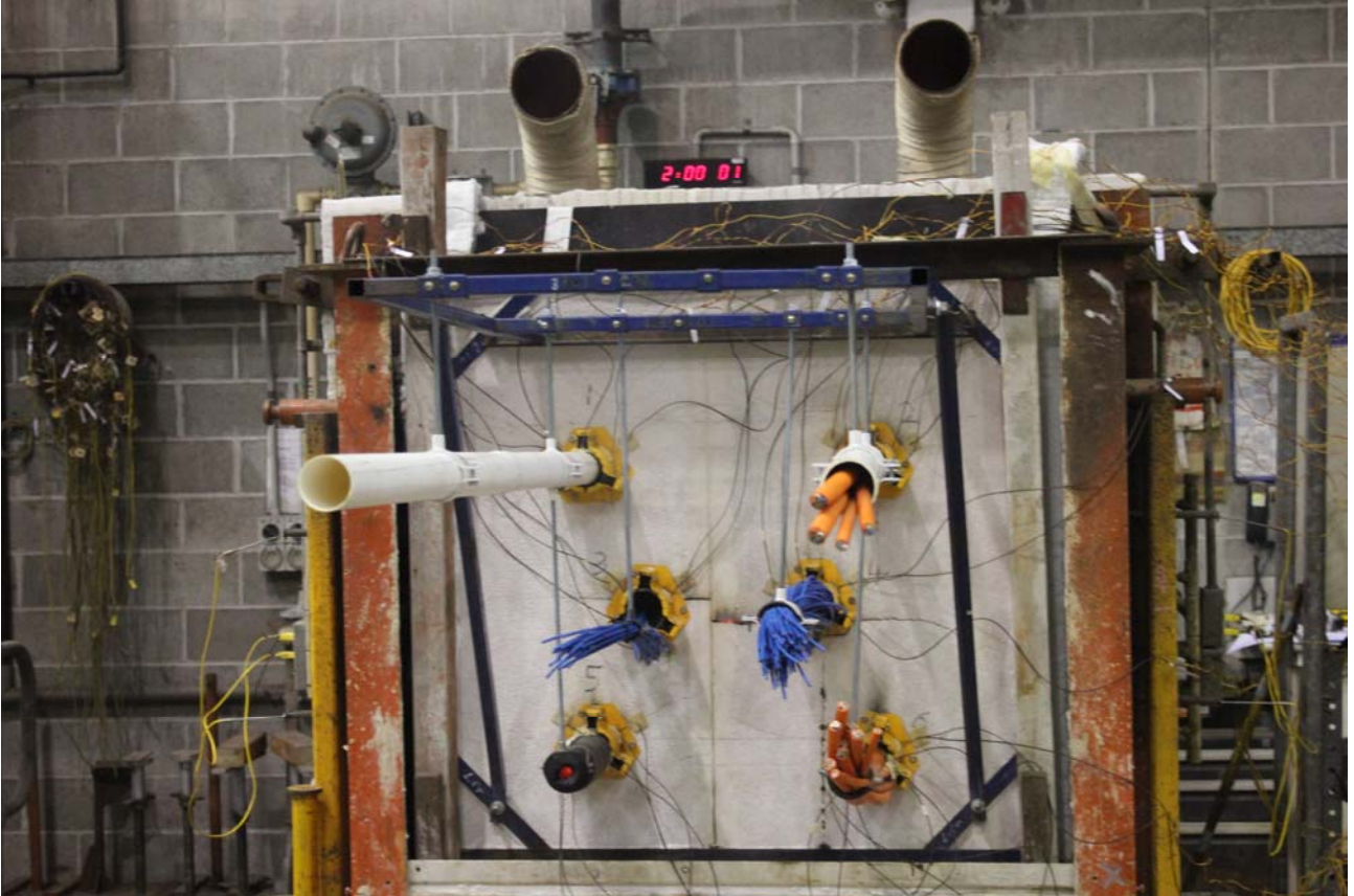
PHOTOGRAPH 12 – SPECIMENS AFTER 120 MINUTES OF TESTING
