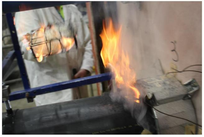
PHOTOGRAPH 17 - COTTON PAD TEST APPLIED TO SPECIMEN 3 AFTER 153 MINUTES OF TESTING
