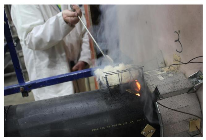
PHOTOGRAPH 16 - COTON PAD TEST APPLIED TO SPECIMEN 3 AFTER 153 MINUTES OF TESTING
