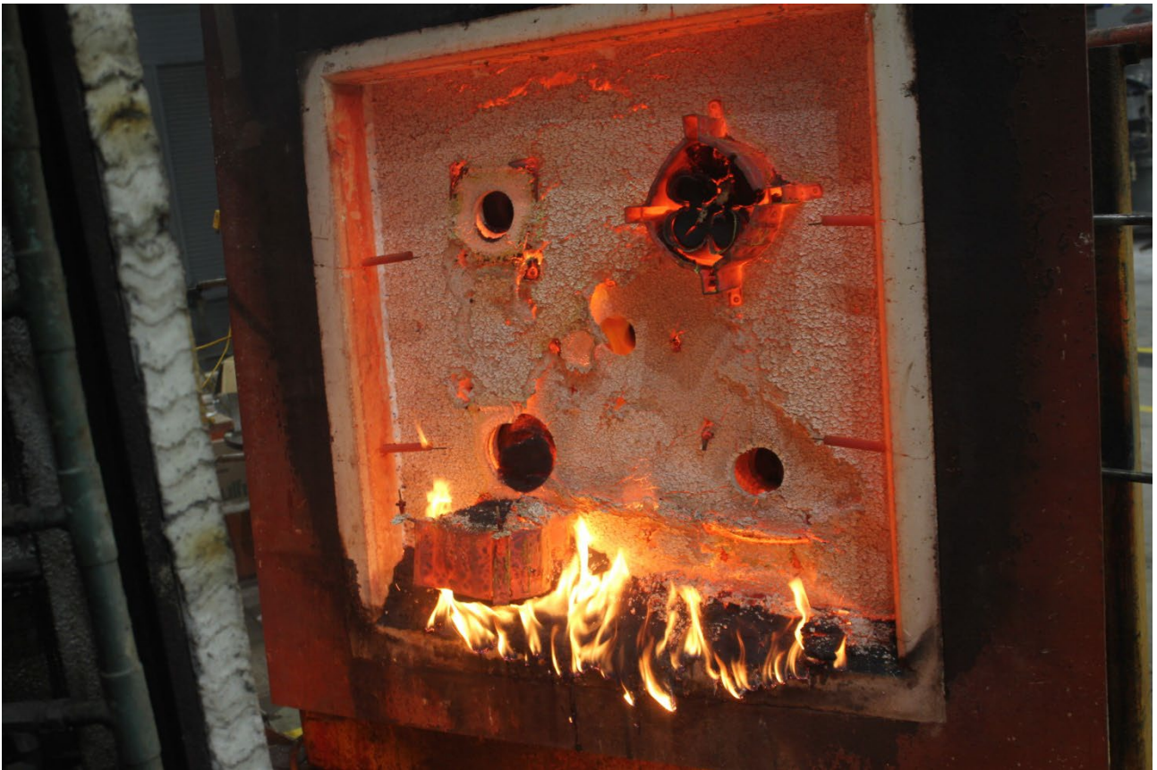
PHOTOGRAPH 19 – EXPOSED FACE OF SPECIMENS AT CONCLUSION OF TESTING
