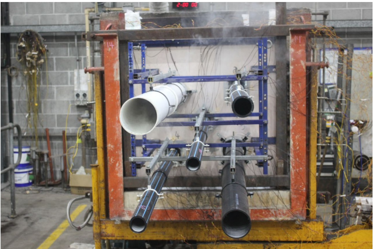
PHOTOGRAPH 12 –SPECIMENS AFTER 120 MINUTES OF TESTING
