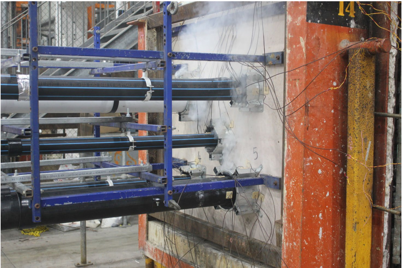
PHOTOGRAPH 13 –SPECIMENS AFTER 131 MINUTES OF TESTING
