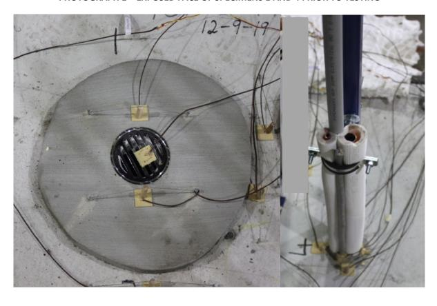
PHOTOGRAPH 2 – UNEXPOSED FACE OF SPECIMENS 1 AND 4 PRIOR TO TESTING
