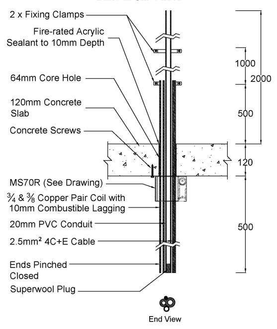
DRAWING TITLED "SPECIMEN #4 ¾-IN AND A ¾-IN INSULATED COPPER PAIR COIL, 20 PVC CONDUIT, 3 CORE CABLE + E & MS70R", DATED 12 SEPTEMBER 2019, PROVIDED BY SNAP FIRE SYSTEMS PTY LTD
