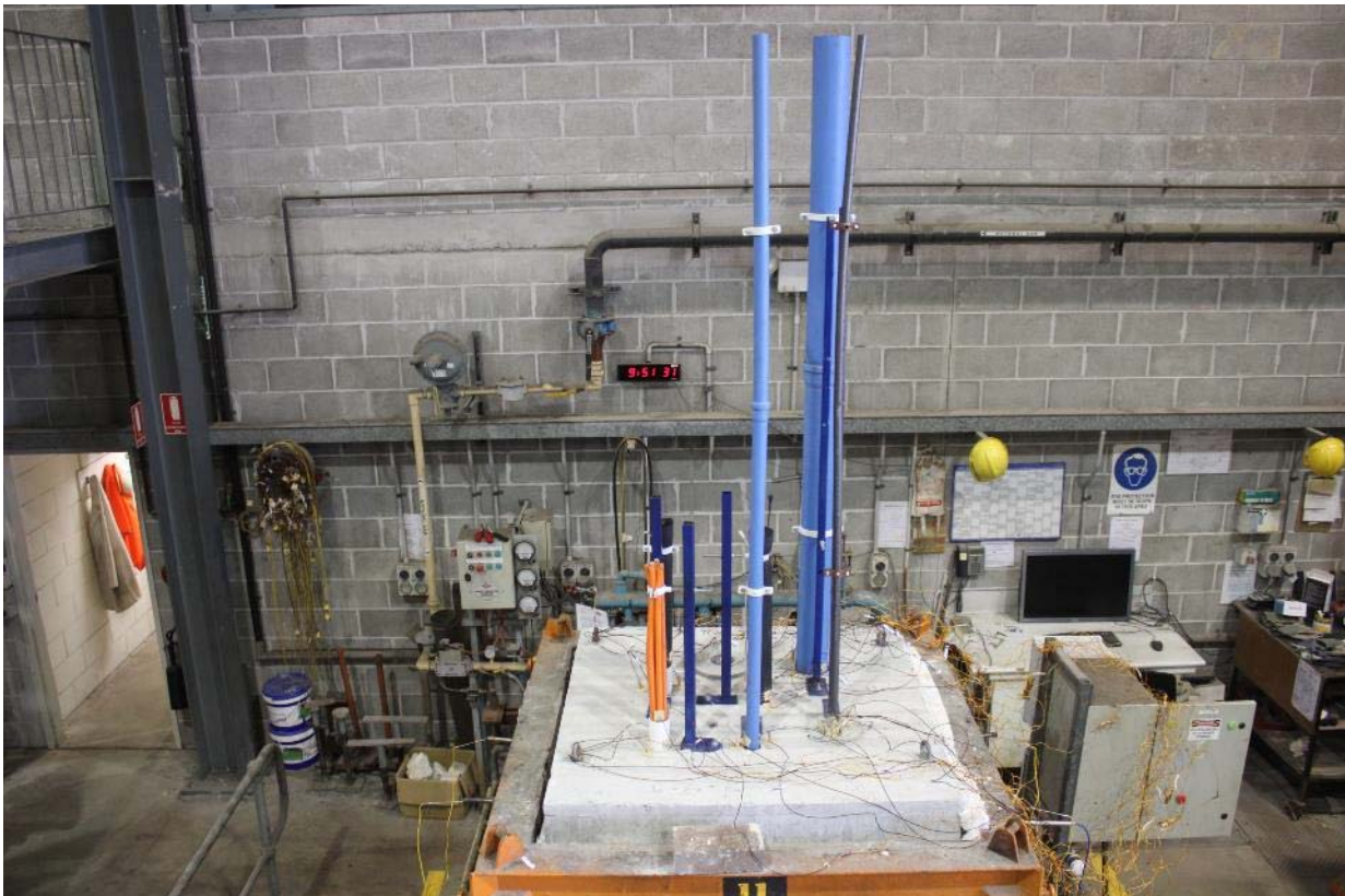
PHOTOGRAPH 2 – UNEXPOSED FACE OF SPECIMENS PRIOR TO TESTING
