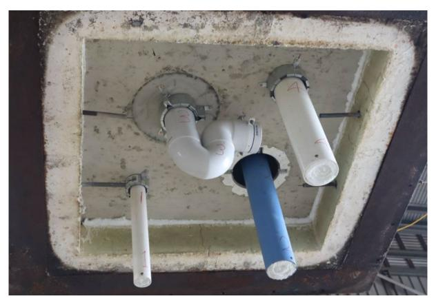
PHOTOGRAPH 1 – EXPOSED FACE OF SPECIMENS PRIOR TO TESTING
