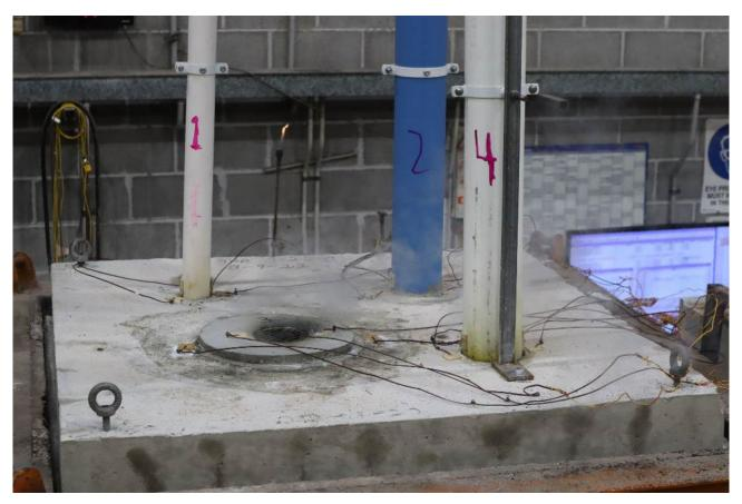
PHOTOGRAPH 10 – TOP VIEW OF SPECIMENS AT 120 MINUTES INTO THE TEST
