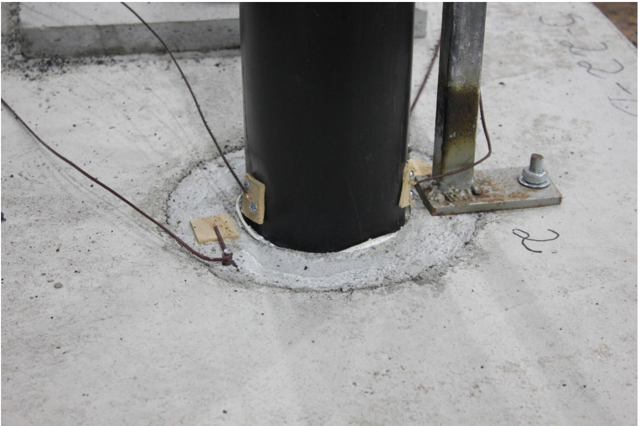
PHOTOGRAPH 13 – THE BASE OF SPECIMEN 2 AT 230 MINUTES INTO THE TEST
