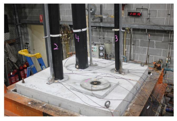
PHOTOGRAPH 10 – SPECIMEN 1 AT 120 MINUTES INTO THE TEST
