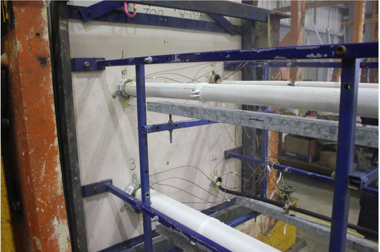
PHOTOGRAPH 8 – UNEXPOSED FACE OF SPECIMENS AT THE CONCLUSION OF TESTING
