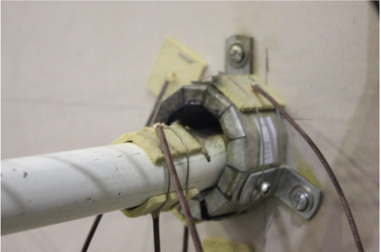
PHOTOGRAPH 6 – SPECIMEN 2 AFTER 54 MINUTES OF TESTING
