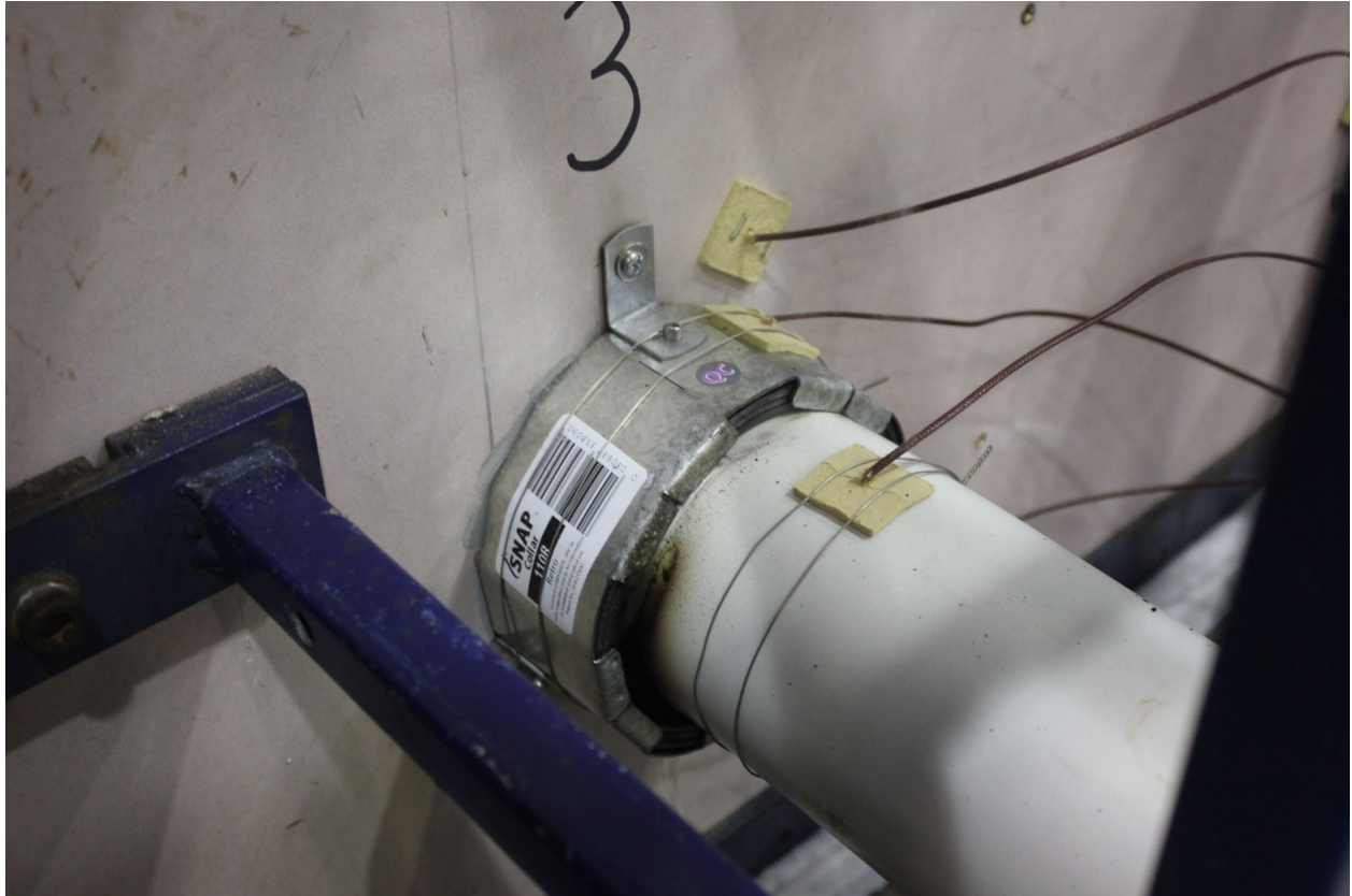
PHOTOGRAPH 4 – SPECIMEN 3 AFTER 31 MINUTES OF TESTING
