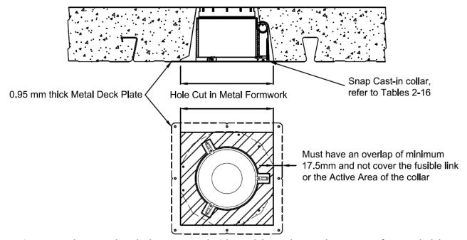
Figure 19: When Metal Deck Plates are used with Bondek or other steel permanent formwork slab
