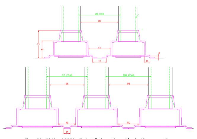
Figure 33a: CC 40 and CC 50 collar installation options with min. 40mm separation
