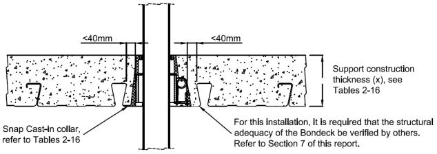
Figure 17: An example of the installation of SNAP collars in concrete with Bondek slab only – an active area of the collar < 40mm from the edge of the deck rib
