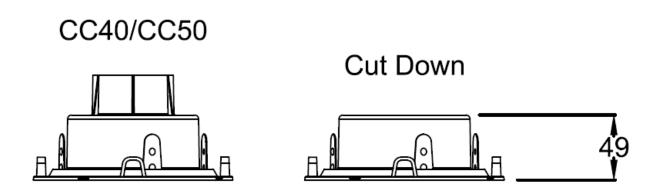
When the top of the collar is cut down lower than the top of the slab depth, the gap between the top of the collar and the pipe must be sealed with a bead of sealant or PVC tape to prevent the ingress of concrete slurry into the Active Area of the collar
