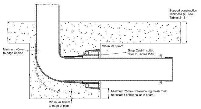
Figure 14: Examples of a horizontal orientation on the side of a beam
