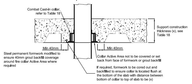
Figure 29: An example of the installation of Combat Collars in concrete with Bondek or other steel permanent formwork slab – an active area of the collar ≥40mm from the edge of the deck rib
