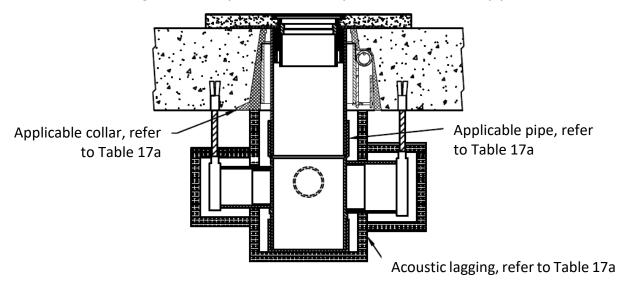
Figure 25: Example of acoustic wrap on floor waste PVC/HDPE pipes
