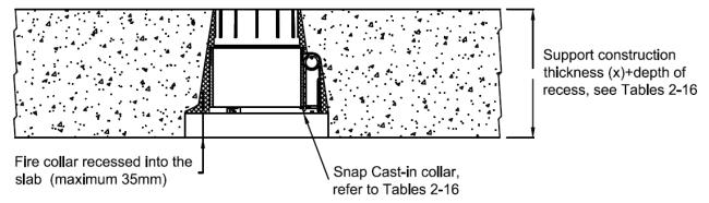
Figure 21: Examples of fire collar recessed
