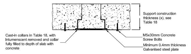
Figure 36: Sealing method of empty Cast-In collars
