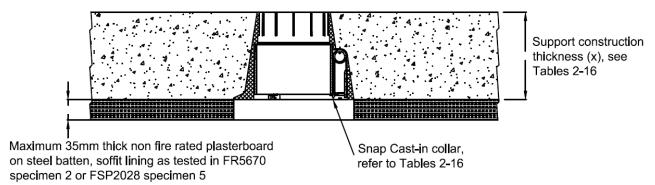
Figure 22: Examples of slab soffit lining opening for the fire collar
