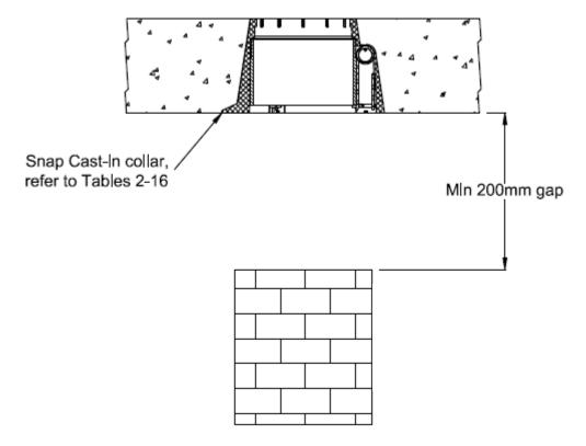
Figure 15: Examples of fire collar recessed
