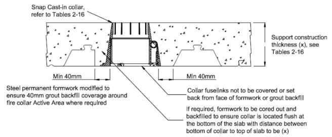
Figure 16: An example of the installation of SNAP collars in concrete with Bondek or other steel permanent formwork slab – an active area of the collar ≥40mm from the edge of the deck rib
