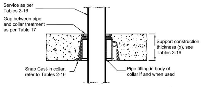
Figure 6: Example of installation of SNAP Cast-In collars with stack pipes in concrete slab/concrete with Bondek or other steel permanent formwork slab
