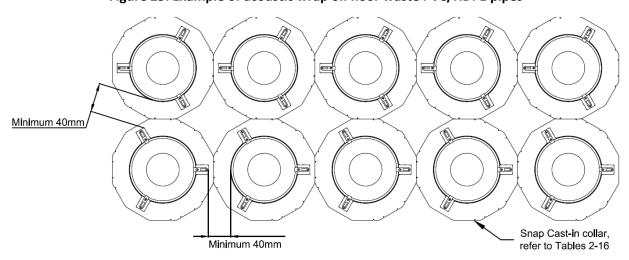
Figure 25a: Examples of collars in a cluster with stack pipes – Min. 40mm between the active area of collars
