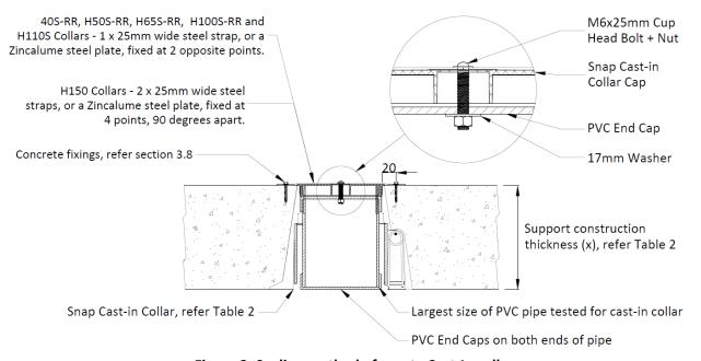
Figure 8: Sealing method of empty Cast-In collars
