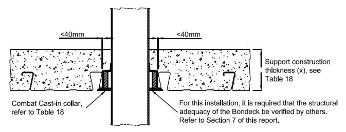
Figure 30: An example of the installation of Combat Collars in concrete with Bondek slab only – an active area of the collar < 40mm from the edge of the deck rib.
