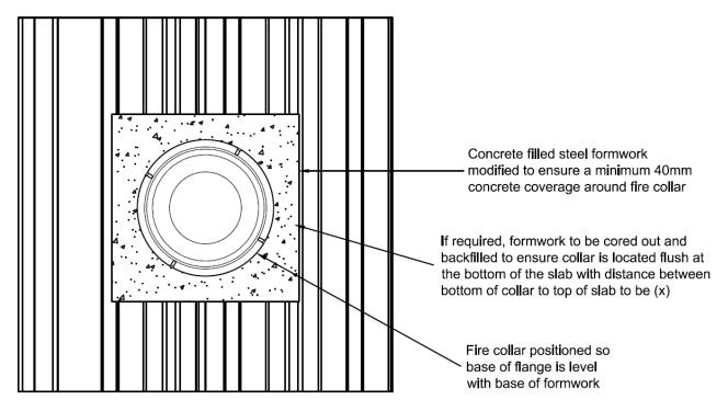
Figure 31: Base of Cast-In collar flange level with the base of Bondek or other steel permanent formwork slab
