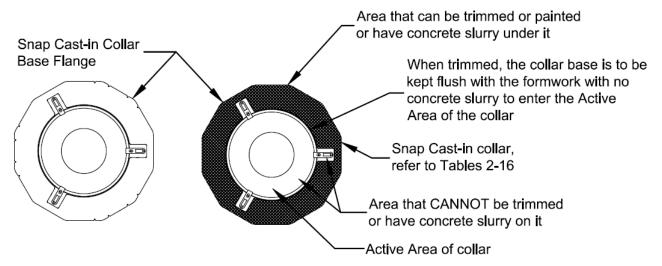
Figure 10: Definition of areas that can be trimmed or painted or have slurry under
