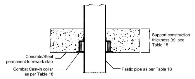
Figure 28: Installation of Combat collars with stack pipes in a concrete slab, Bondek or other steel permanent formwork slab
