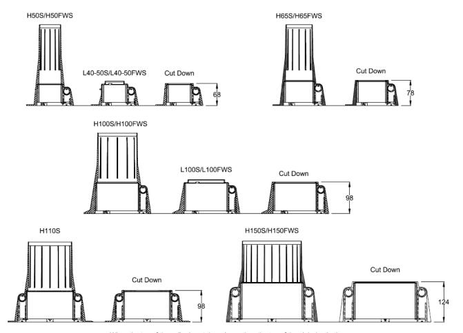
When the top of the collar is cut down lower than the top of the slab depth, the gap between the top of the collar and the pipe must be sealed with a bead of sealant or PVC tape to prevent the ingress of concrete slurry into the Active Area of the collar
