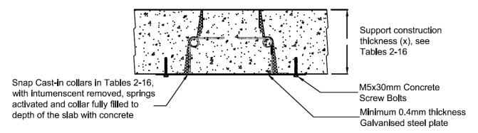
Figure 9: Sealing method of empty Cast-In collars
