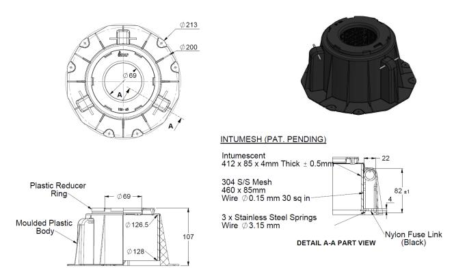
Figure 2f: SNAP L65FWS collar (L100FWS with a 65mm reducer ring)
