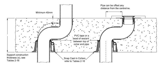
Figure 13: Examples of cast-in pipework above cast-in collar configuration
