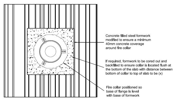
Figure 18: Base of Cast-In collar flange level with the base of Bondek or other steel permanent formwork slab
