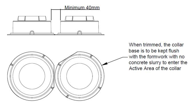
Figure 33: Examples of collar separation and example of the extent of flange trimming (Refer to Figures 33a and 33b for section view)
