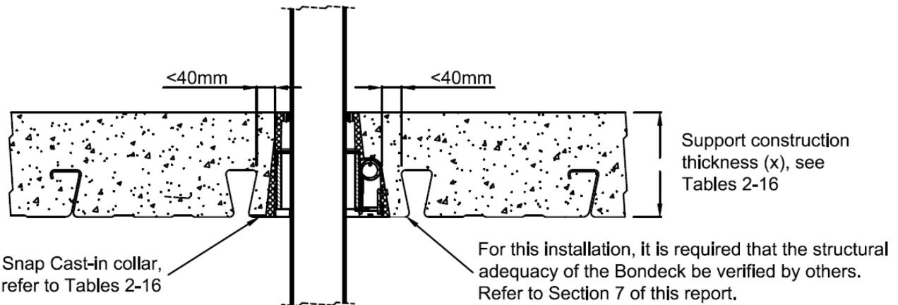
**Figure 17: An example of the installation of SNAP collars in concrete with Bondek slab only – an active area of the collar  $< 40\text{mm}$  from the edge of the deck rib**
