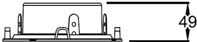
When the top of the collar is cut down lower than the top of the slab depth, the gap between the top of the collar and the pipe must be sealed with a bead of sealant or PVC tape to prevent the ingress of concrete slurry into the Active Area of the collar
