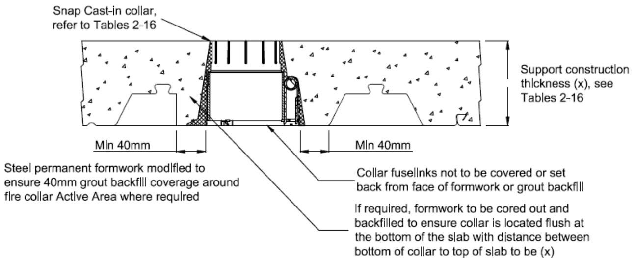
**Figure 16: An example of the installation of SNAP collars in concrete with Bondek or other steel permanent formwork slab – an active area of the collar  $\geq 40\text{mm}$  from the edge of the deck rib**
