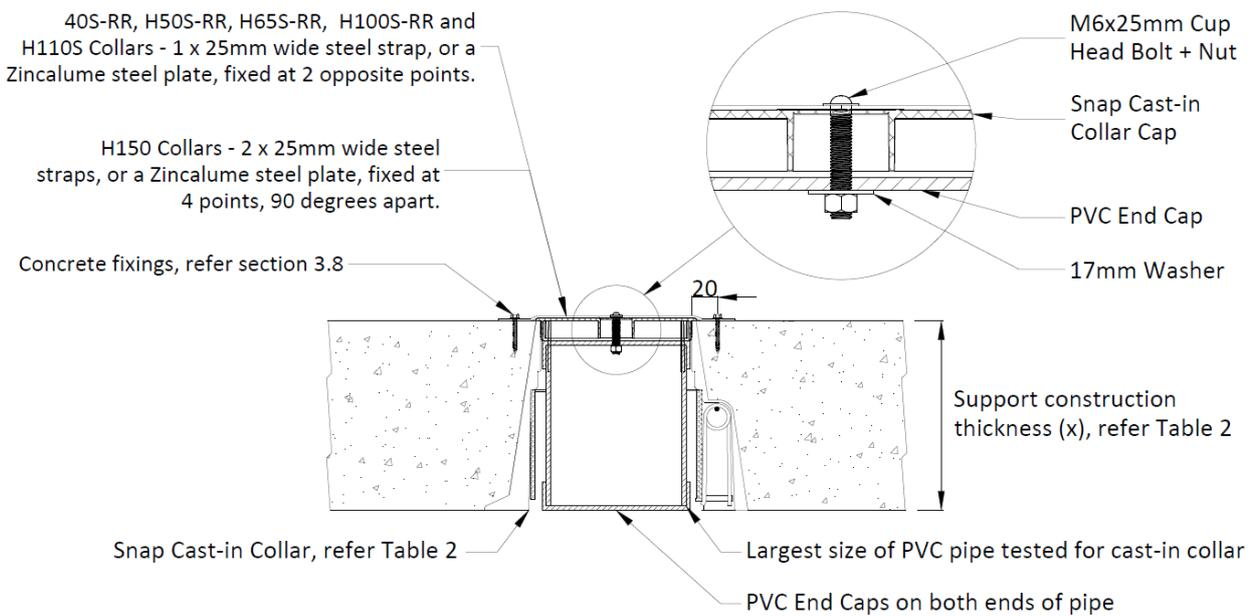
**Figure 8: Sealing method of empty Cast-In collars**
