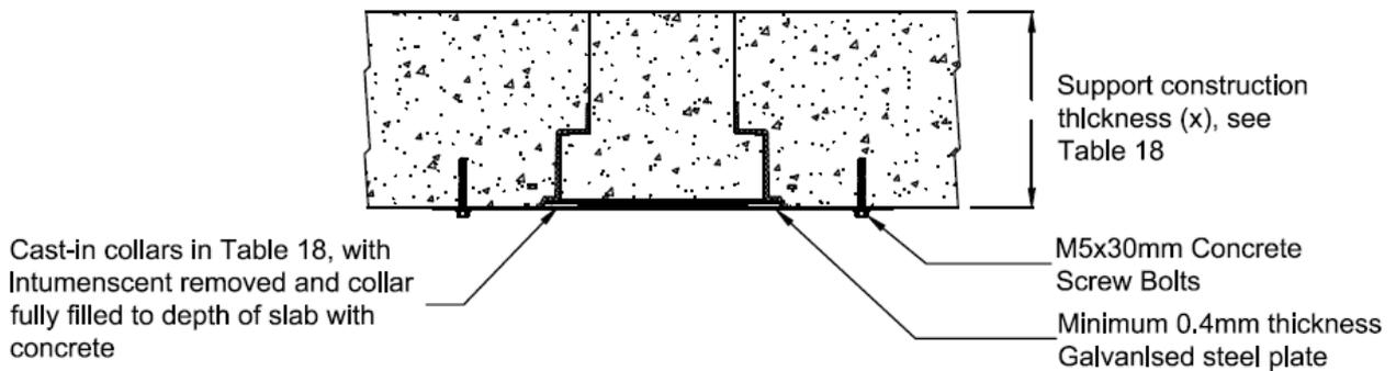
**Figure 36: Sealing method of empty Cast-In collars**
