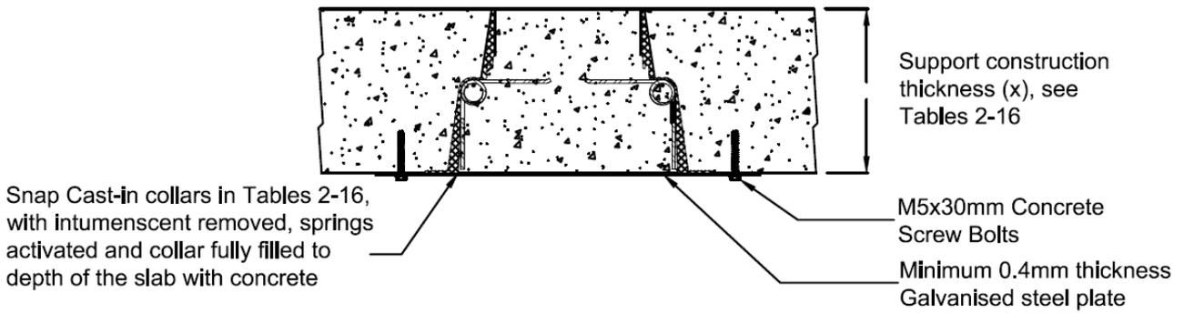
**Figure 9: Sealing method of empty Cast-In collars**
