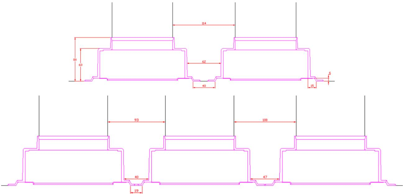
Figure 33b: CC 100 collar installation options with min. 40mm separation
