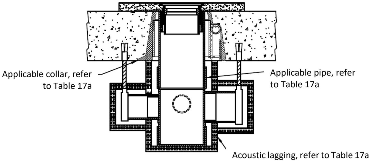
**Figure 25: Example of acoustic wrap on floor waste PVC/HDPE pipes**
