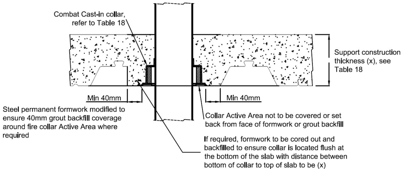
**Figure 29: An example of the installation of Combat Collars in concrete with Bondek or other steel permanent formwork slab – an active area of the collar  $\geq 40\text{mm}$  from the edge of the deck rib**
