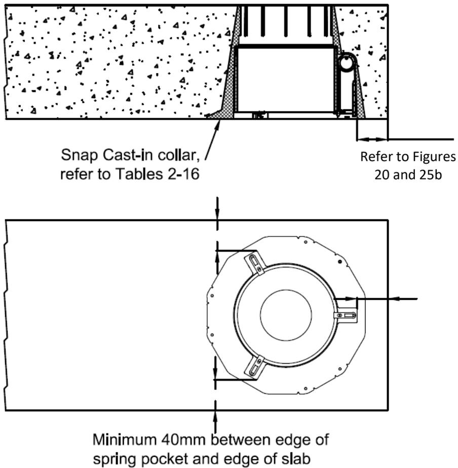
**Figure 20: Cast- in collar with stack pipes when 40mm from the slab edge**
