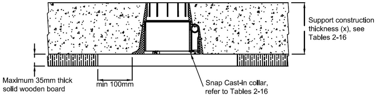
**Figure 23: Examples of slab soffit lining opening for the fire collar**
