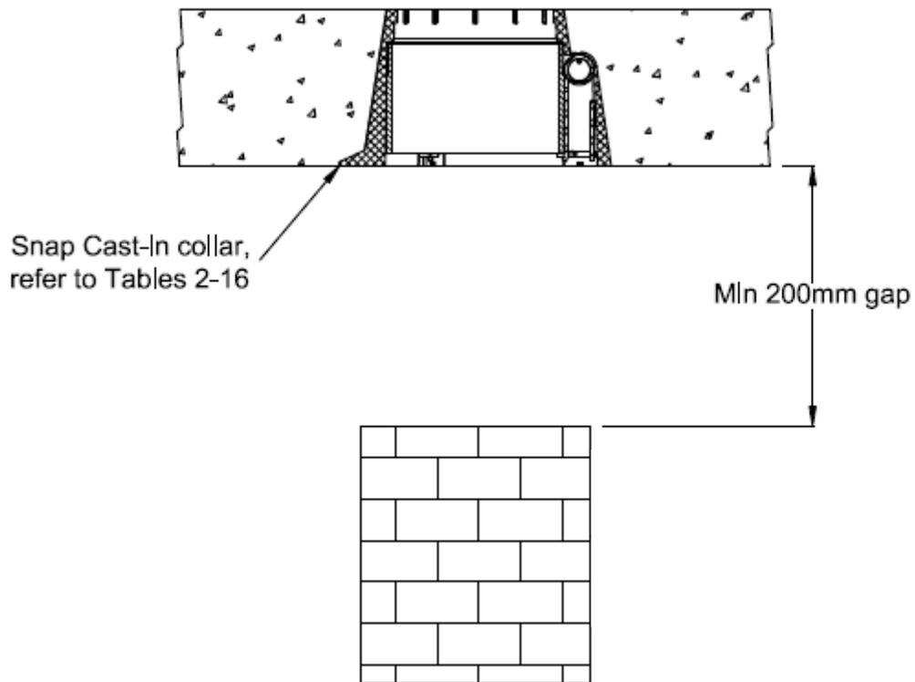
**Figure 15: Examples of fire collar recessed**
