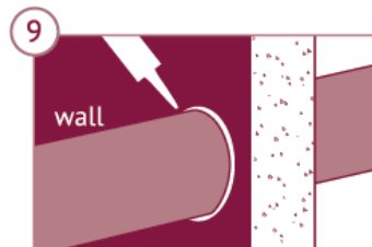
9 Seal annular gap between the wall and pipe on both sides as required (see Table 3)
