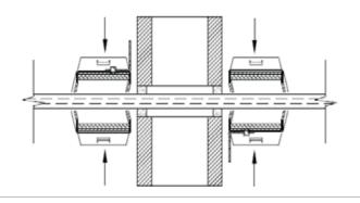
Fasten the collar to the element using appropriate fixings through all circular holes in the base plate.
