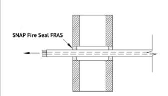
Wrap the collar around the services and close, ensuring both clasps are engaged. Slide the collar against the wall or underside of the slab.
